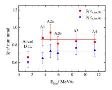
Figure 7: Normalised transverse emittances at different beam energies.
