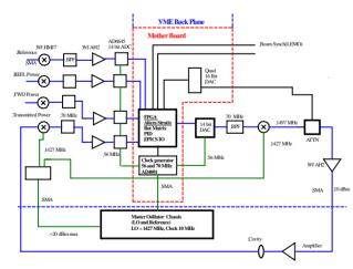
Figure 2: RF system block diagram.
