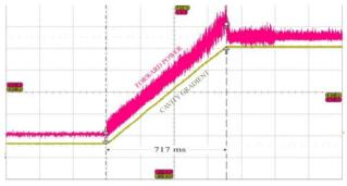
Figure 3: Graph of gradient and forward power as RF is turned on.
