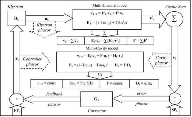
Figure 2: Algebraic model of LLRF control system.
