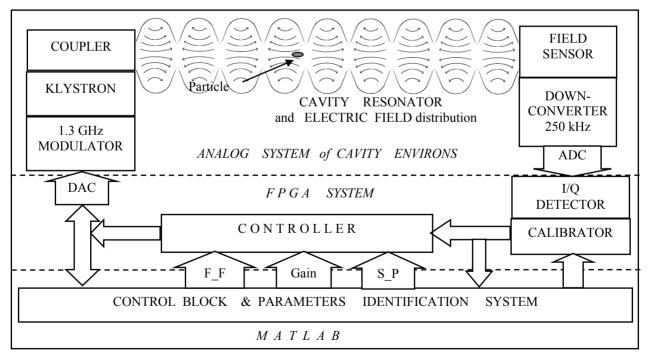
Figure 1: Functional block diagram of low level radio frequency cavity control system.
