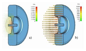
Figure 2: Microwave Studio 3D model of a DTL type cavity: a) Electric Field Vector, b) Magnetic Field Vector.
