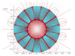
Figure 5: OPERA 2D plot of a PMQ with 16 wedges of material, and an integrated printed-circuit quadrupole.
