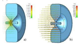
Figure 3: Microwave Studio 3D model of a CCL type cavity: a) Electric Field Vector, b) Magnetic Field Vector.
