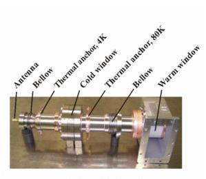
Figure 2: Assembled coupler.
