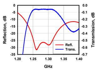
Figure 3: Measured passband of single coupler.
