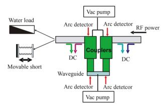
Figure 4: Scheme of high power test.
