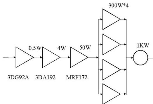
Figure 2: 1kW Solid-state exciter combined by four MRF151G 300W preamplifiers.
