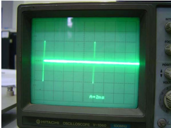
Figure 6: The output sample of 487kW RF signal with 100 $\mu$ s pulse duration and duty cycle 1%.
