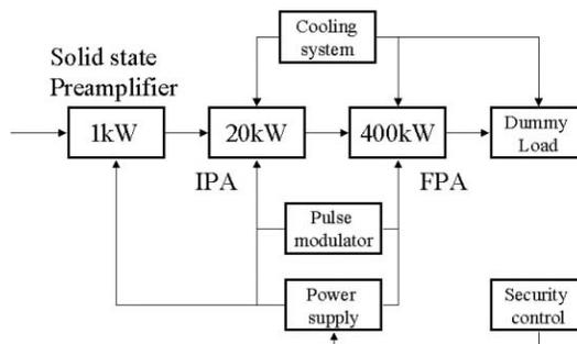
Figure 1: Schematic diagram of 400kW amplifier.
