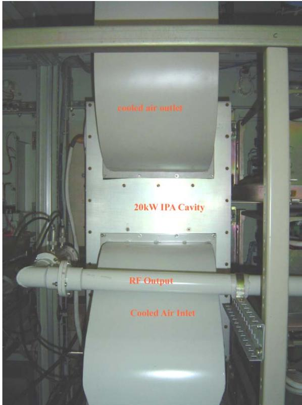
Figure 3: FU113F 20kW IPA cavity.
