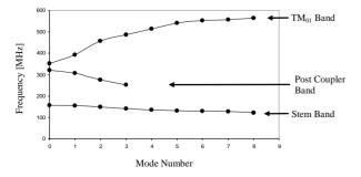
Figure 2: Computed mode frequencies in 1/3 of Tank 1.
