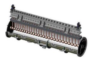
Figure 3: 3D open view of DTL Tank1 prototype [4].
