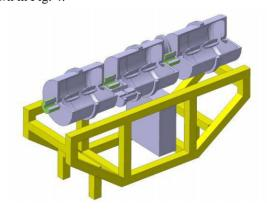
Figure 4: 3D cut-away view of the first CCDTL module.
