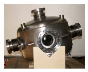
Figure 1:  $\beta$  0.15 spoke with its helium tank.
