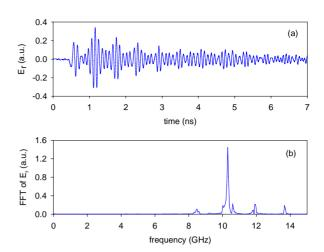
Figure 6: Measurement of the radial electric field driven by an 86 nC electron bunch, using the field probe on Structure 3: (a) temporal profile of the radial electric field; (b) the FFT of the signal.
