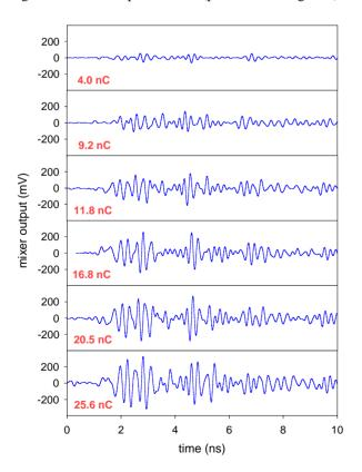
Figure 2: Output of RF mixer for various bunch charges that propagated through Structure 1.
