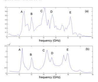
Figure 5: FFT of the radial component of the electric field (in arbitrary units), identifying the peaks A, B, C, D, E, respectively, as the modes  $\text{HEM}_{111}$ ,  $\text{TM}_{012}$ ,  $\text{TM}_{013}$ ,  $\text{HEM}_{112}$ ,  $\text{TM}_{014}$ : (a) measurement; (b) MAFIA simulation, taking into account the measured Q factor of each mode.
