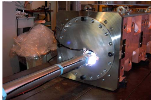
Figure 3: LBW processing the cavity inside.
