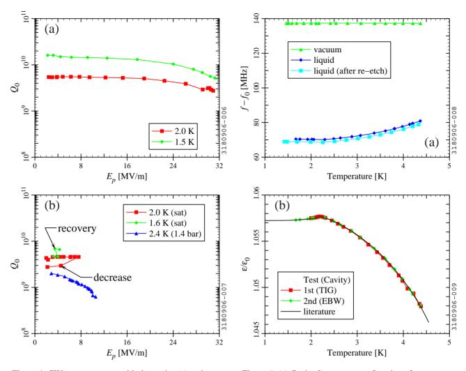
Figure 4. CW measurements with the cavity (a) under vacuum and (b) filled with liquid helium.
