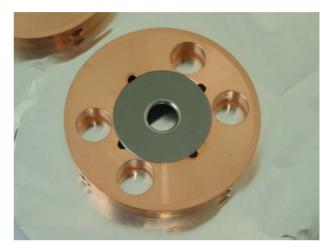
Figure 1: Tungsten-iris inserted into a copper disk forming together a cell of the rf structure. The beam aperture is 9.2 mm.
