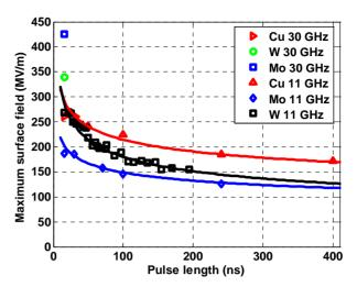
Figure 3: Pulse length dependence of the maximal surface field for different structures.
