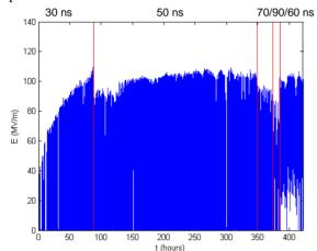
Figure 2: Conditioning history of the tungsten-iris structure in NLCTA.
