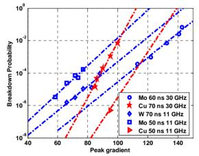
Figure 4: Break down probability as a function of gradient, for different structures.
