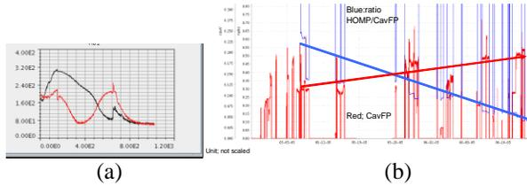
Figure 3: Change of waveform through HOM feedthrough at the same operating gradient (long term changes).
