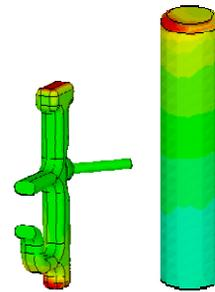
Figure 6: Electric field distributions at HOM coupler feedthrough and inner conductor of fundamental power coupler from stray field coupling of cavity fundamental mode frequency.
