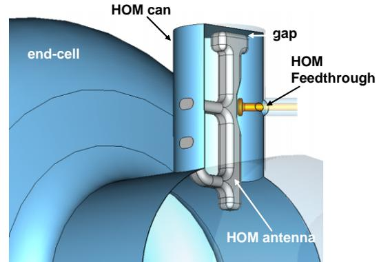
Figure 1: SNS SRF cavity assembly and HOM coupler.
