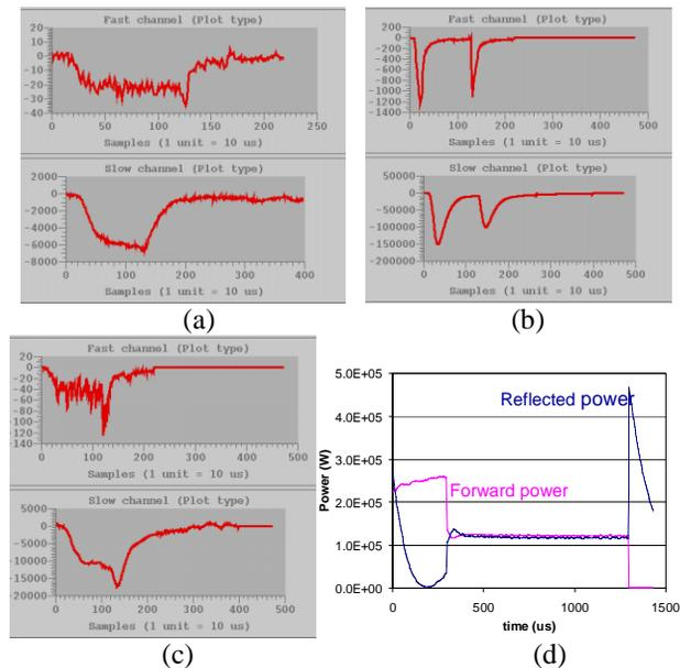
Figure 7: Radiation patterns from cavity. (a) cavity field type, (b) full traveling wave type, (c) combined type and (d) waveforms of forward and reflected power in closed loop.
