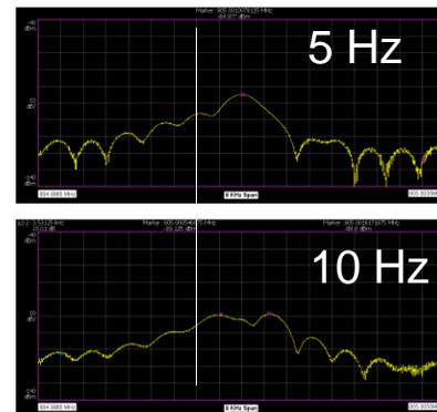
Figure 8: spectrum analyzer measurement of signals from HOM feedthrough with RF only at 5 and 10 Hz. The vertical line corresponds to the resonance frequency of the cavity tested.
