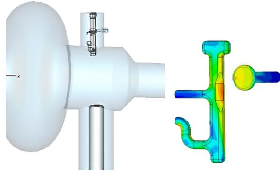
Figure 5: MWS modeling and magnetic field distributions at HOM antenna and feedthrough from stray field coupling of cavity fundamental mode frequency.
