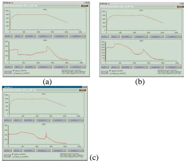
Figure 4: Repetition rate dependent waveforms through HOM coupler. (a) waveform at 1 to 5Hz, (b) waveform at 30 Hz, and (c) waveform at 30 Hz 20 min. after the repetition rate is set to 30 Hz.
