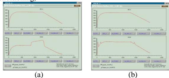
Figure 2: Abnormal waveforms through HOM feedthrough running RF only without beam (electron loading). (a) at 3.5 MV/m, (b) at 6 MV/m.
