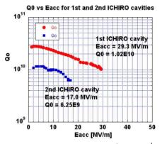
Figure 5: Vertical test results for 1st and 2nd ICHIRO cavities.
