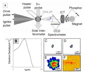
**Figure 1.** (A) Experimental setup showing the gas jet with laser beams and diagnostics. (B) The density profile of the channel obtained by Abel inversion of the side interferogram. (C-F) Mode images of laser propagation at 4 TW. The output image with the guide on (D) is indistinguishable from the input (C) indicating unaberrated propagation at twice  $P_{crit}$ . Unguided images show diffraction in vacuum (E) and ionization enhanced diffraction with the gas jet on (F).
