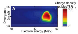
**FIGURE 2.** Electron bunch. The electron energy spectrum of the channeled accelerator shows the appearance of monoenergetic features, here with  $2x10^9$  electrons in a bunch with energy spread of 4% FWHM at 86 MeV. Divergence was near 3 mrad FWHM.
