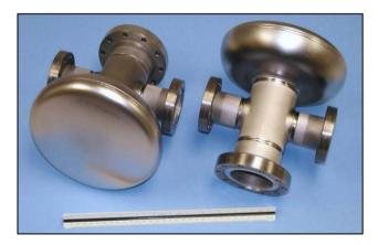
Figure 1: GHz SRF <sup>1</sup>/<sub>2</sub> Cell Guns.
