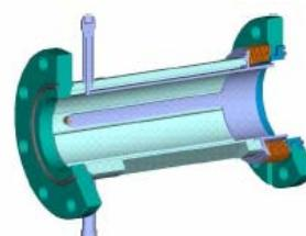
Figure 2: Cutaway BPM assembly.
