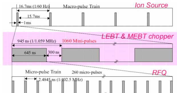
Figure 1: SNS bunching and gap structure. [1]
