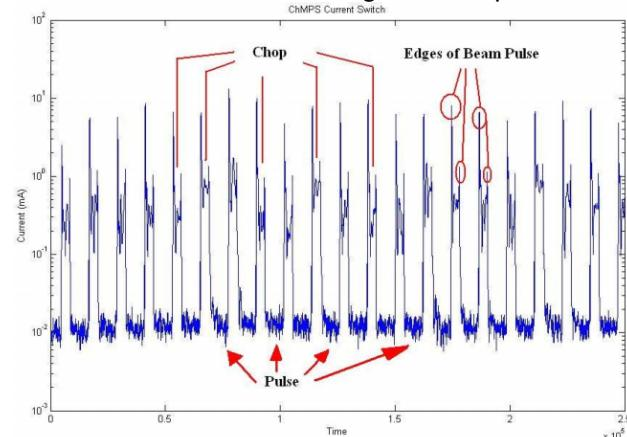
Figure 8: ChMPS with timing switch analyzing beam gaps.
