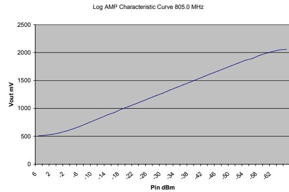
Figure 5: Log Amp characteristic curve.
