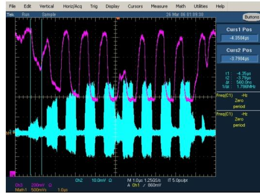
Figure 6: ChMPS measurement of a mini-pulse with failed chopper.
