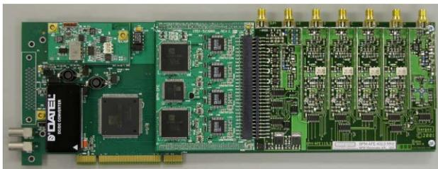
Figure 1: The custom PCI BPM data acquisition card.
