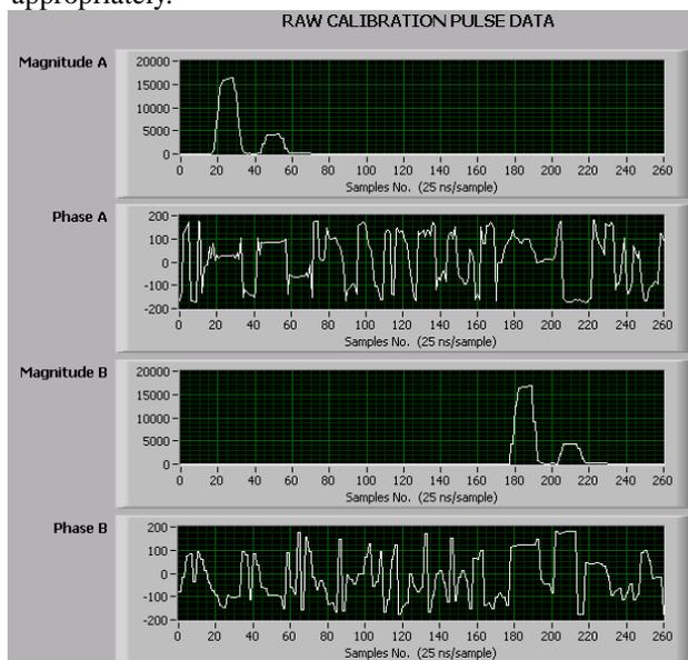
Figure 3: Typical calibration waveforms seen within the LabVIEW® application for two of the four channels. Note that the phase signals are random noise without the presence of a calibration signal pulse.
