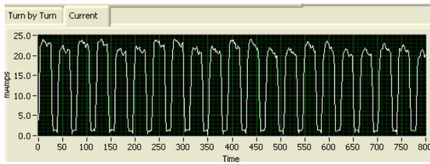
Figure 5: The BPM system is also used as a beam current monitor as there are few beam current transformers in the linac.
