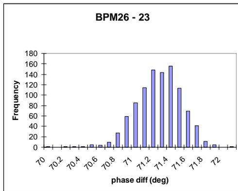
Figure 6: A typical histogram of the differential-phase measured between two BPMs whose electronics are in the same rack are. The data is 1000 beam pulses, averaged over 20  $\mu$ s. The jitter is 0.26 degrees rms.
