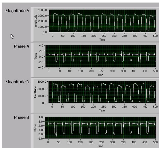
Figure 4: Actual beam signals for two lobes within a position pickup. The ratio of magnitudes would be processed to give the position measurement. The beam is chopped for injection into the storage ring.
