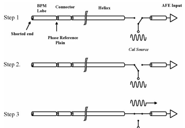
Figure 2: The calibration uses an rf burst to calibrate the down converter chain in step 1, launch a calibration burst down the BPM Heliac® cable in step 2 and measure the reflected burst in step 3.
