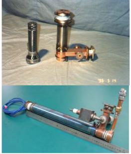
Figure 2: X-band accelerating tubes, 2.5MeV (upper) and 6MeV (lower).
