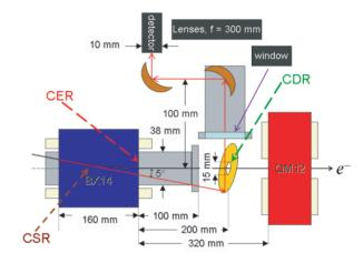
Figure 1: Layout of the LCLS bunch length monitor BL11.
