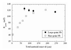
Figure 5: Maximum value of  $B_p$  at 2 K as a function of material removal for the large grain single cell used for this study compared with the results from a previous study [5] done on a fine grain cavity.
