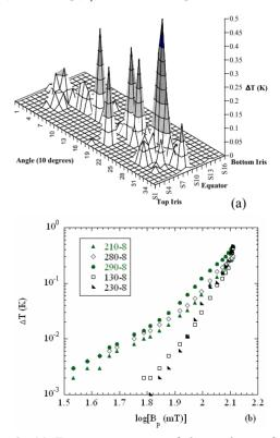
Figure 3: (a) Temperature map of the cavity surface at 1.7 K and  $B_p = 126$  mT after 95  $\mu$ m of total material removal and (b)  $\Delta$ T vs. log( $B_p$ ) for few "hot-spots".
