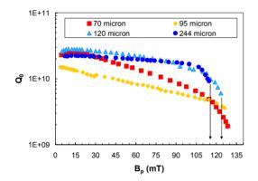
Figure 1:  $Q_0$  vs.  $B_p$  at 1.7 K as a function of the total material removal.
