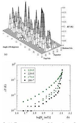
Figure 2: (a) Temperature map of the cavity surface at 1.7 K and  $B_p = 128$  mT after 70 µm of material removal and (b)  $\Delta T$  vs. log( $B_p$ ) for few "hot-spots".
