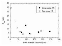
Figure 4: Residual resistance as a function of material removal measured on a fine grain [5] and on a large grain Nb cavity at 1.5 GHz.
