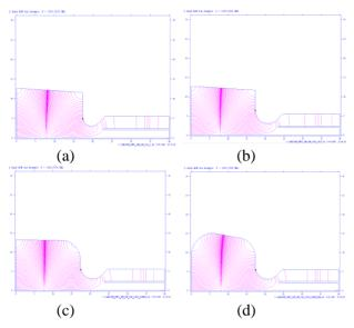
Figure 1: Design examples for an HOM RF gun: (a) with an output iris radius of 2.4 mm; (b) with an output iris radius of 3.4 mm; (c) with a rounding radius of 5 cm on the outer cell wall at the output end; and (d) with an additional rounding radius of 6 cm.
