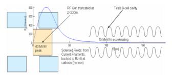
Figure 3: Layout for the beam dynamics simulation.
