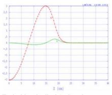
Figure 2: Typical longitudinal (red) and transverse (green) electrical fields distribution along the gun axis.
