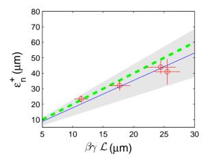
Figure 2: Larger one of the flat beam emittances  $(\varepsilon_n^+)$  versus  $\beta\gamma\mathcal{L}$ . A linear regression (solid line) of the experimental data (circle) is compared with the theoretical dependence (dashed line). The shaded area represents the 95% confidence bounds associated with the linear regression.
