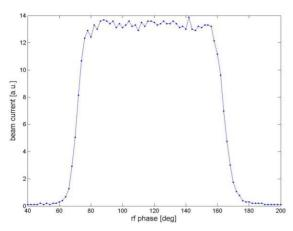
Figure 8: Plot of DTL tank 3 acceptance scan.
