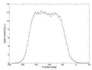
Figure 6: Plot of DTL tank 1 acceptance scan.
