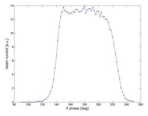
Figure 7: Plot of DTL tank 2 acceptance scan.
