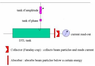
Figure 5: Schematic drawing of acceptance scan with the absorber and collector.
