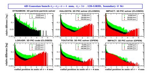
Figure 1: Relative field error for DYNAMION and PIC codes with a grid resolution of 128<sup>3</sup>(129<sup>3</sup>).
