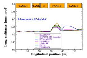
Figure 3: Zero-current simulation: longitudinal RMS emittance computed by all the codes and plotted along the DTL.
