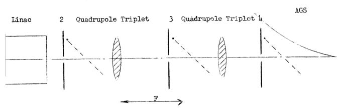
The lens between viewing box 2 and 3 is set so that its focal length equals the distance from the lens to viewing box 3. The observations on screen 3 give the maximum beam divergence. Using now a slit in viewing box 2 and observing again beam spot size on screen 3 will give the divergence of the central rays. The following results were obtained:
