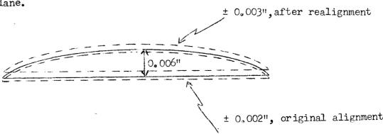
Misalignments in the vertical plane were of the same order of magnitude as those in the horizontal plane, except that the maximum displacements were located near both ends of the Linac. These might have been caused by changes in Linac supports due to the addition of a shielding wall at the high energy end and building excavations in the vicinity of the low energy end.
