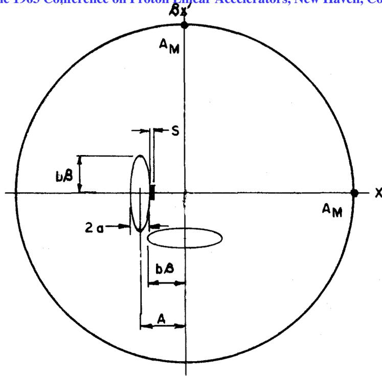
Fig. 3. Accelerator acceptance and beam emittance at injection and on first turn.
