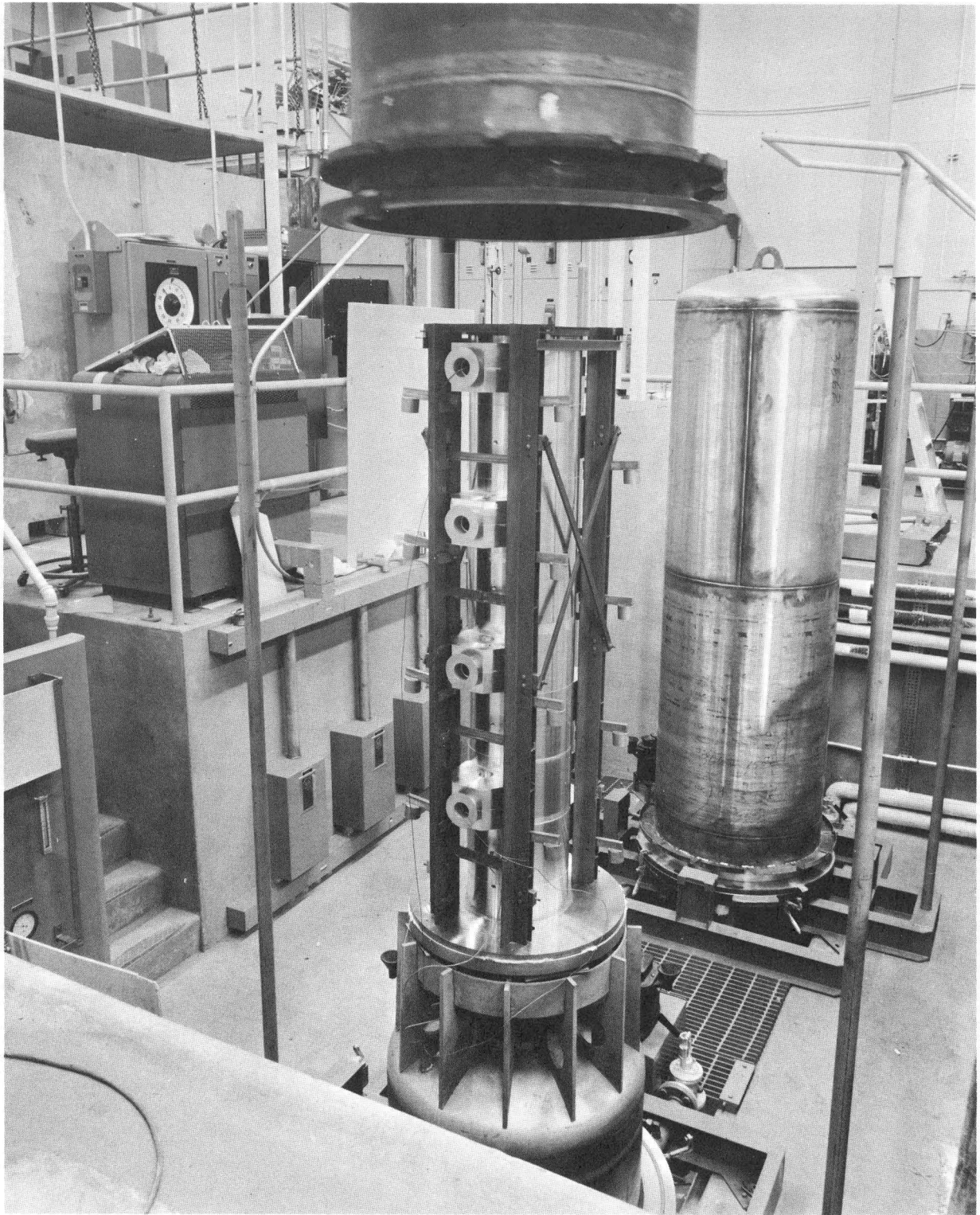
Figure XI - Tank Section in Furnace for Final Heat
