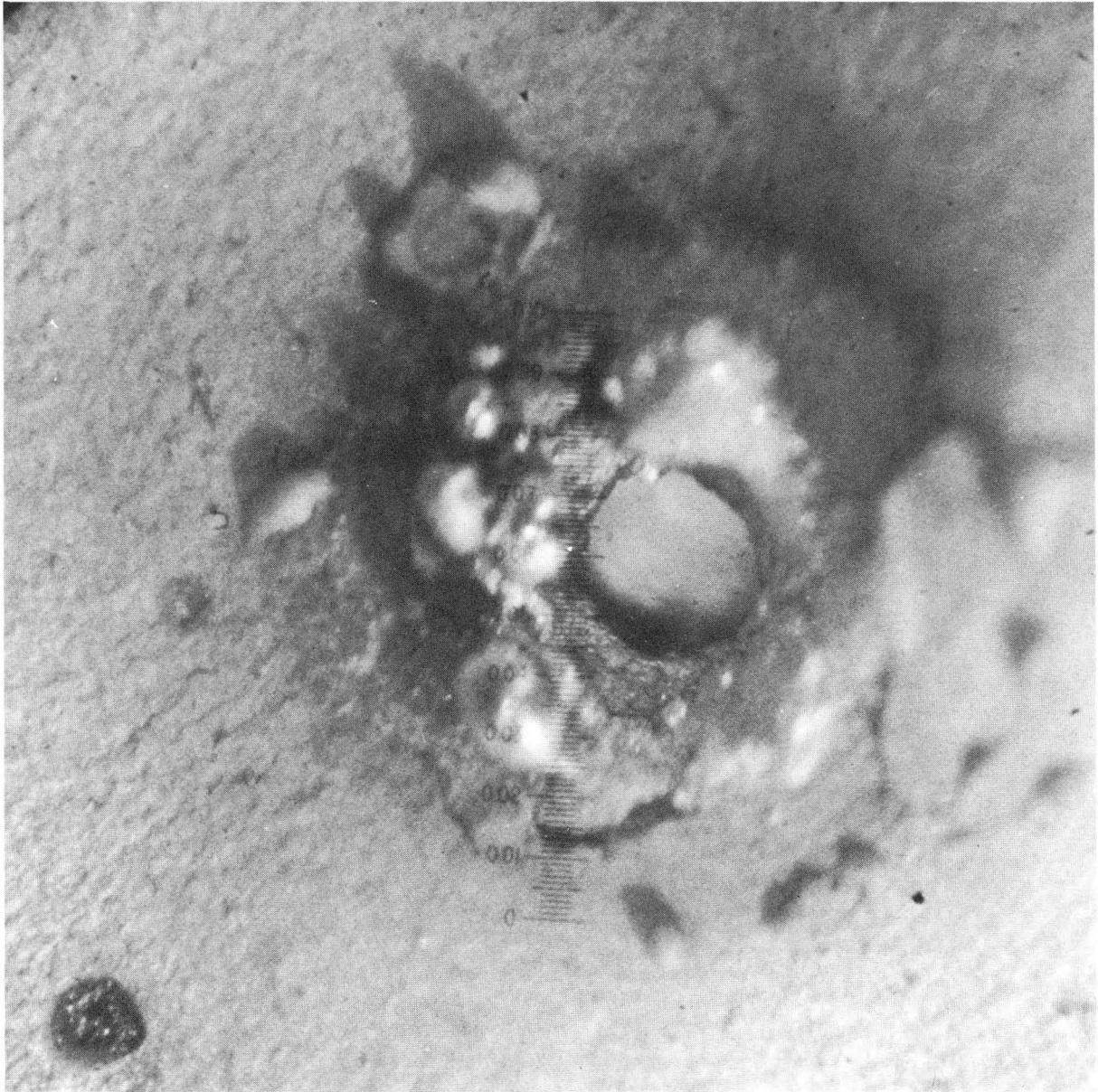
Fig.12. Photomicrograph of plasma aperture from the intermediate electrode side after 12% duty factor life test.
