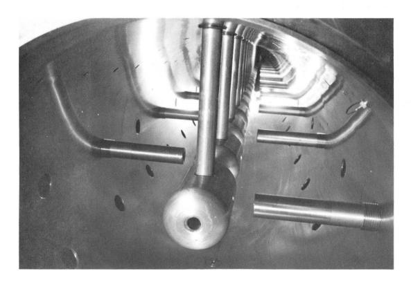
Fig.1. Post Coupled Drift Tube Linac Structure
