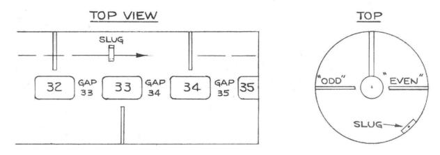
Fig.3. Experimental Setup for Measurement of Relative Post Excitations
