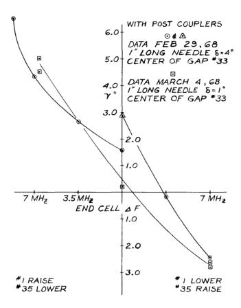
Fig.9. Comparison of Transverse Field Data Taken with Needles of Different Misalignments
