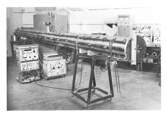
Fig.2. 35-Cell Post Coupled Drift Tube Linac Model
