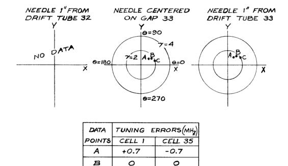
Fig.11. Polar Plot of Transverse Field Data for Structure without Post Couplers
