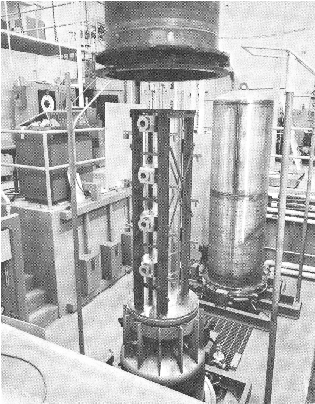
Figure 21. An EPA Tank in Place for Final Braze Operation
