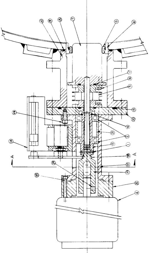
Fig. 9. Motorized tuner -- cavity 1.
