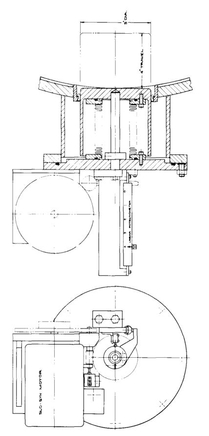
Fig. 8. Motorized tuner -- cavity 2 through 9.
