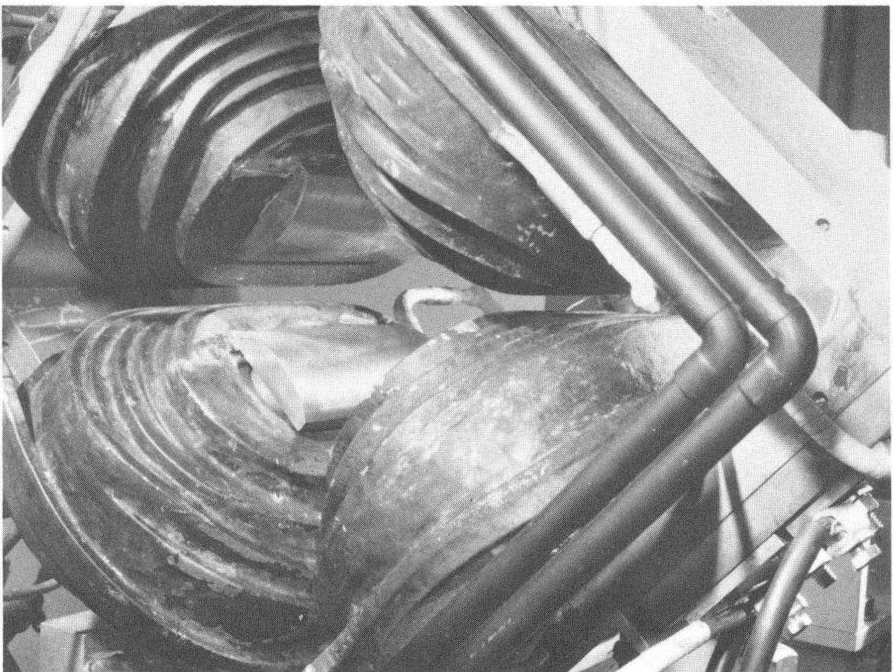
Fig. 2. 4-in. bore quadrupole wound with solid conductor, m.i. cable, externally cooled.
