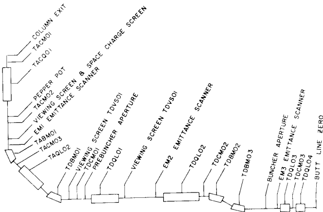
Fig. 1b. Schematic diagram of the high-intensity proton-beam line.
