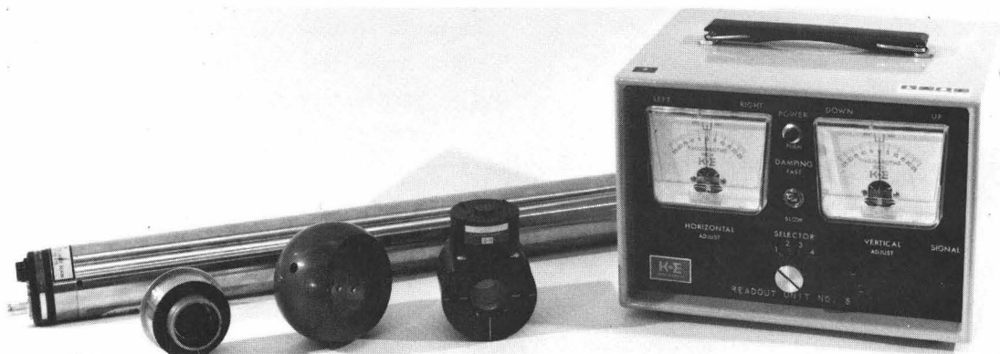
Fig. 1. Commercial tooling laser system used to align LAMPF.
