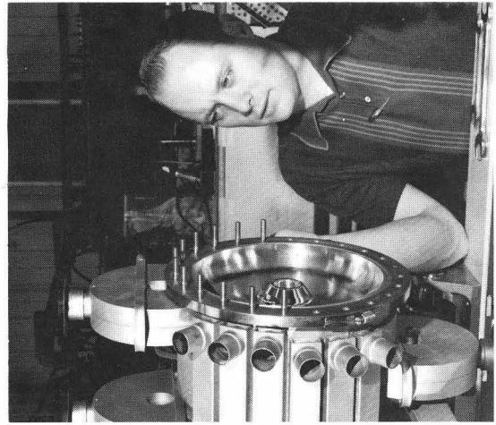
Fig. 14 Preparation and inspection 805 MHz tank joint
