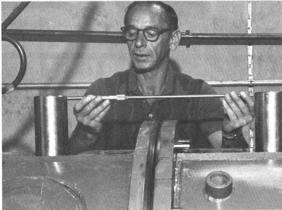
Fig. 5 Drift tube spacing measurement 201 MHz tank section joint
