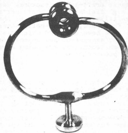
Fig. 5: 240 MHz superconducting split-ring element developed at Cal Tech. The ring is fabricated from chemically polished Pb electroplated onto copper. The diameter of the ring is 12.6 cm, the diameter of the ring tubing is 0.95 cm, and the diameter of the housing is 25 cm.
