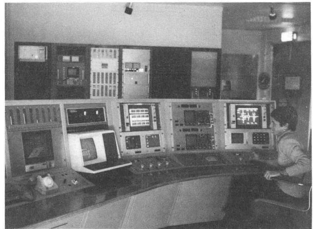
Fig. 3 Photo of the right half of the Main console. The three nearest bays represent the Maxiconsole, interfaced to the Main computer. Thereafter follows the Analogue Console and the Midiconsole, both interfaced to the Front End Computer.
