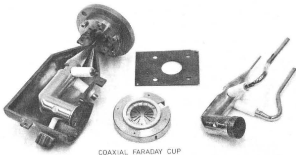
Fig. 4 Coaxial 50 ohm Faraday cup (left). The beam entrance with radial grid (center bottom); isolator protection (top center); inner conductor with cooling water connections (left).
