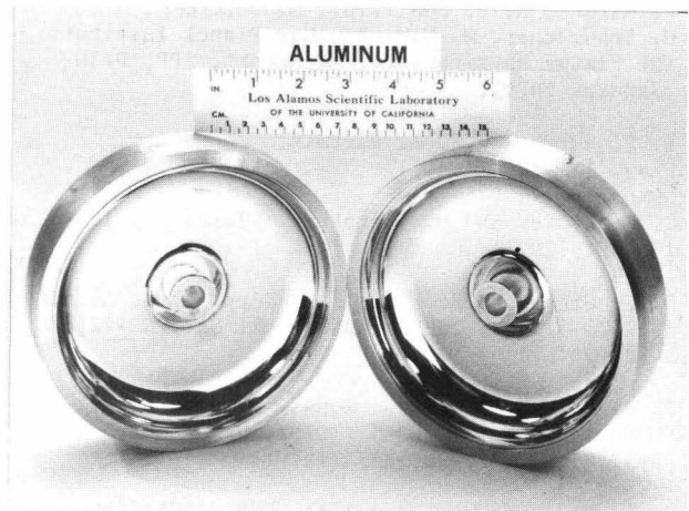
Fig. 2. 1350-MHz Aluminum Segments -- Bright Copper Plated
