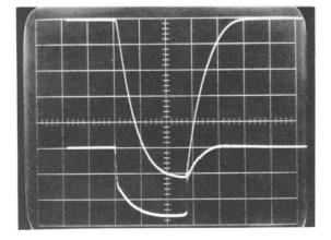
Fig. 1 Upper: rf level in the tank Lower: TH516-II rf output power Horizontal: 100 µsec/div
