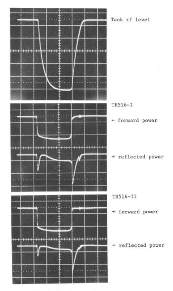
Fig. 8 Waveforms using isolators
