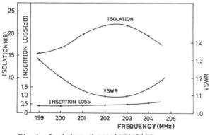
Fig.4 Isolator characteristics
