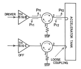
Fig. 5 High power test setup
