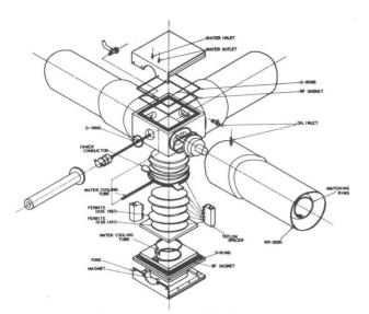
Fig.2 Circulator assembly drawing
