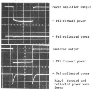
Figure 6 shows the Pf1/Pr1 and Pf2/Pr2 wave shapes. Without correction, their respective scalings may be in error by as much as 10%. Since only relative measurements were made, insertion loss could not be calculated. However, from the circulator surface temperature rise of about 1°C, with an average power of 6 kW, it is clear that insertion loss will not be a problem in normal operation. Also, it is thought that the isolation should be the same as in the low level tests.
