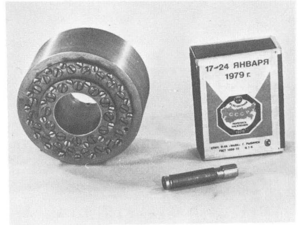
Fig. 5 Rod-type, two-layer, samarium-cobalt quadrupole lens
