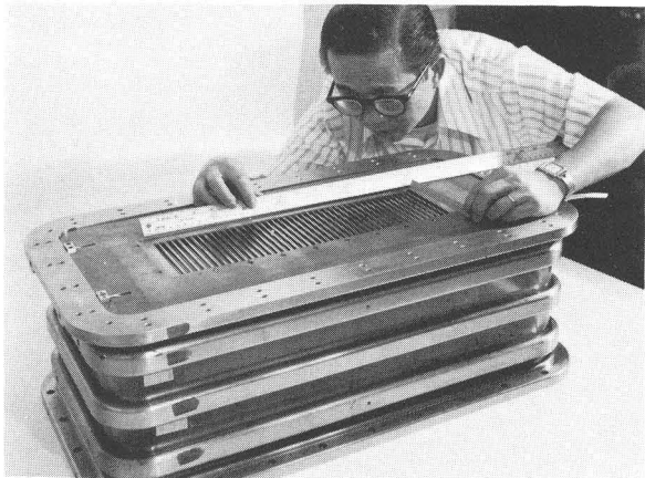
Fig. 8 LBL 120-keV, 65A source, showing extraction slot plates.
