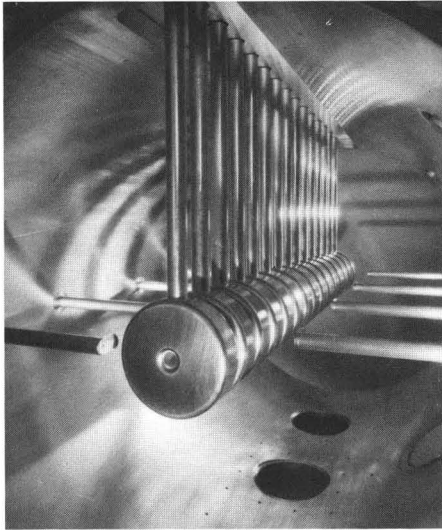
Fig. 1. Photograph of the FMIT scale-model DTL.
