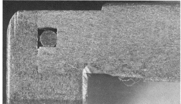
Fig. 1 25 kV combined weld/braze. Disc at top joined to cylinder.
