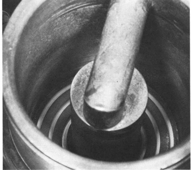
Fig. 3 Alvarez linac loop after ion bombardment damage.
