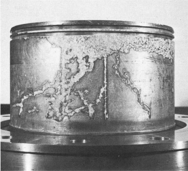
Fig. 2 Surface pitting from rf sparking between loop and port walls.
