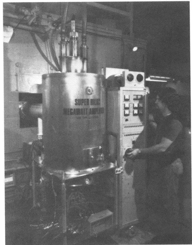
SuperHILAC amplifier with 4CW25K driver.
