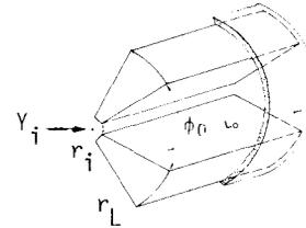
Fig. 3: One RFQ Resonator
