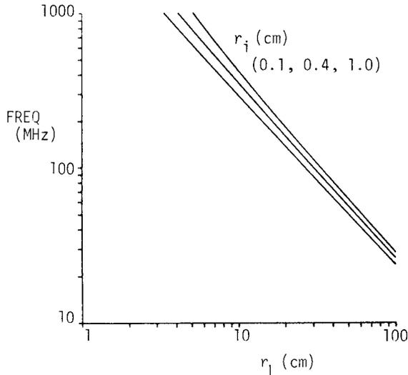
Fig. 5: RFQ Frequency vs.  $r_L$
