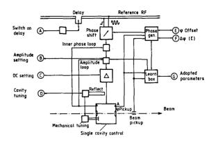
Fig. 7 Block diagramme of the single cavity control system
