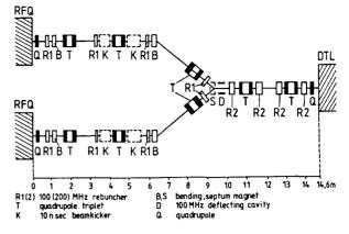
Fig. 3 Concept of the funneling section
