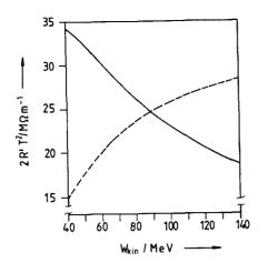
Fig. 4 Shunt resistance of the Alvarez (----) structure, including stems, and the HELA (---) structure;
