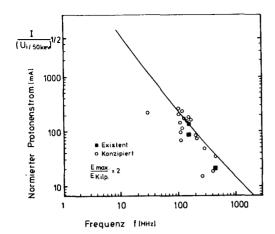
Fig. 2 Maximum RFQ proton current as a function of frequency and injection energy U;
