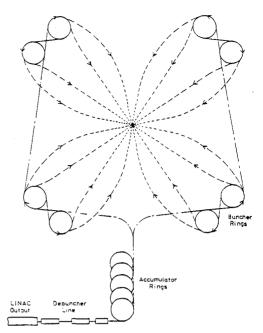
Fig.5 Concept of 4 MJ Driver System at RAL studies by the existing facilities and also accelerator constructions for their purposes are proceeding, as follows. <u>West Germany</u> - Beam and target experiments will be performed on SIS-18 and ESR-9 in GSI.<sup>8</sup> This facility is scheduled for 1988. Figure 6 shows schematic arrangement of this
